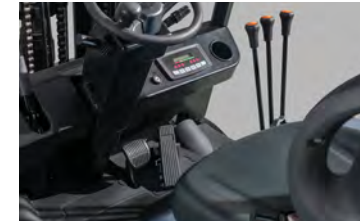
High-visibility display with Indicators and warning lights keeps the operator informed of the forklift's status at a glance.
