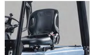
The seat can be adjusted forward and backward and supports a comfortable operating posture by means of side wings and a seat belt.
