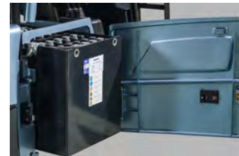
The battery can be taken out from the right side of the truck by using a forklift or pallet truck.
