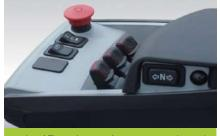
optional Fingertip control system set to rise and fall, forward, backward, lateral and emergency stop switch, a horn, lighting control and other control buttons in one.
