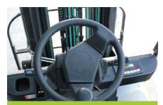
A automobile-like design of the steering wheel and direction switch makes operation more convenient; 3 working modes makes working more efficiently.
